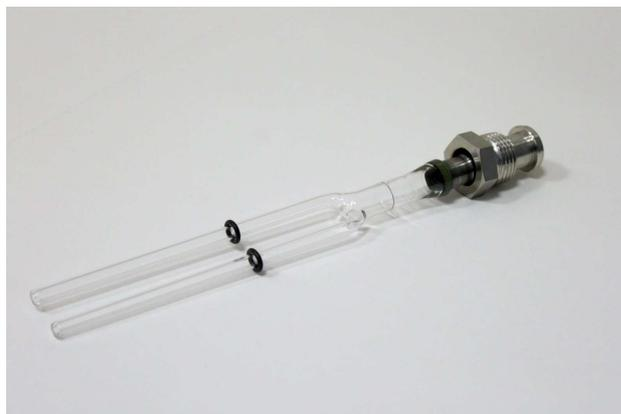
Figure 12 – Silica glass finger and the adaptation to the Sensys DSC
