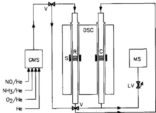
Figure 4 – TC, catalyst; GMS, gas-mixing system; DSC, differential scanning calorimeter; LV, leak valve; MS, mass spectrometer; R, reference; S, sensor; V, valve
