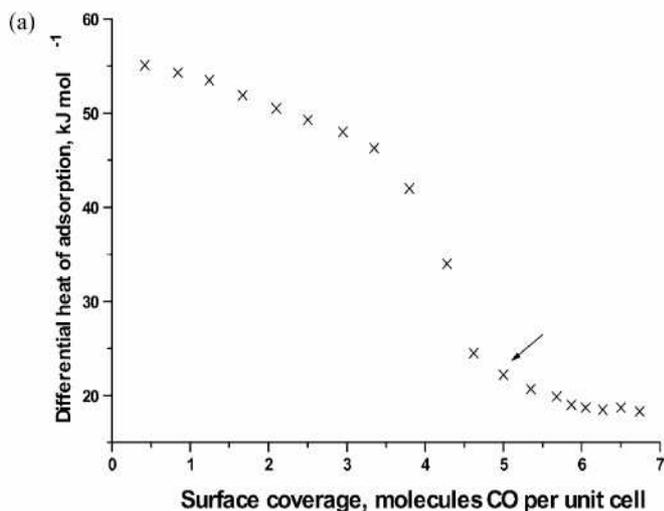
Figure 11 – Differential heats of adsorption of CO on CuY as a function of surface coverage
