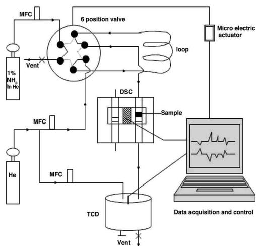
Figure 6 – Pulsed flow adsorption calorimeter system
