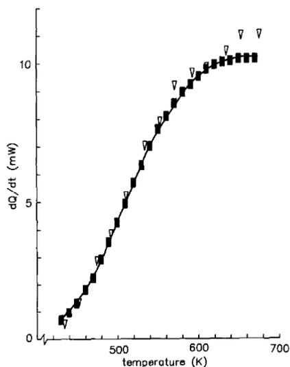
Figure 5 – Heat produced by the reaction of NO, NH<sub>3</sub>, and O<sub>2</sub>, over V<sub>2</sub>O<sub>5</sub> on a TiO<sub>2</sub>/SiO<sub>2</sub> catalyst as a function of temperature
