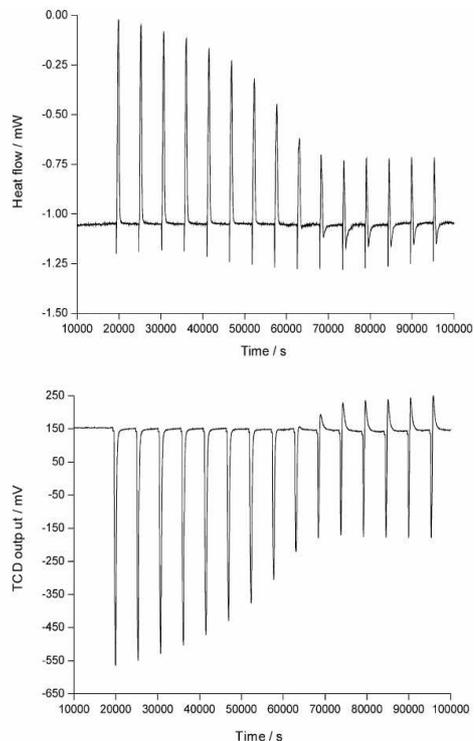
Figure 7 – Typical pulse-FMC data for the ammonia adsorption on Amberlyst 15 at 100 °C and 2ml min<sup>-1</sup> flow rate and corresponding TCD data
