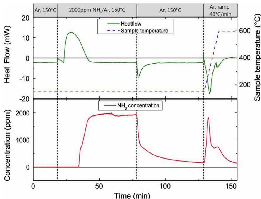
Figure 3 – Thermogram and FTIR signal for an NH<sub>3</sub> TPD experiment on a Cu-Beta catalyst
