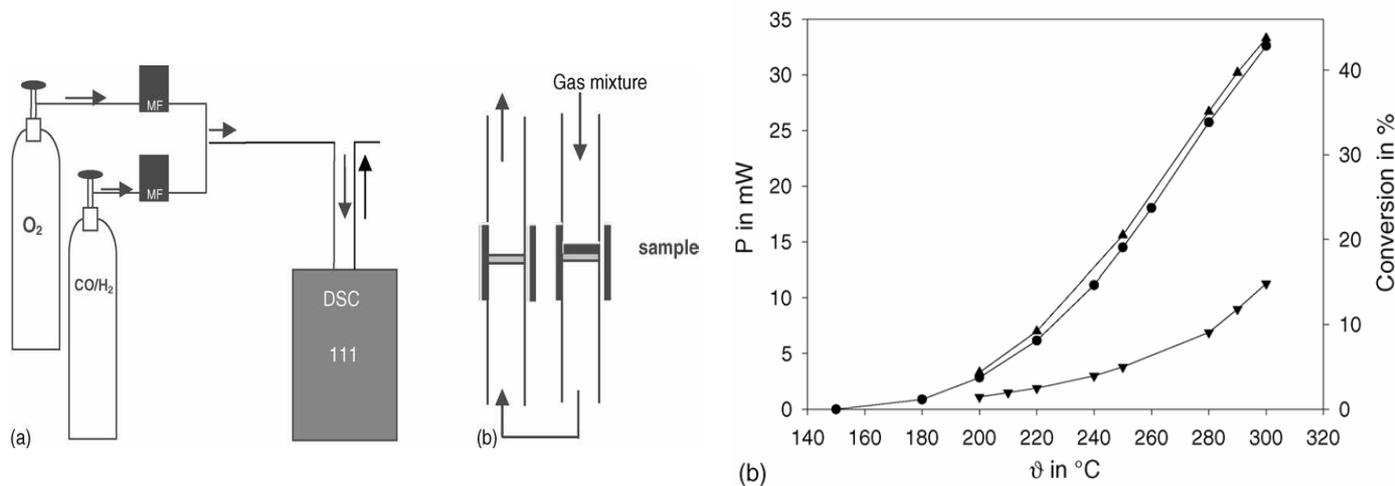
Figure 8 – (a) Mixing of the different gases, (b) Gas flow within the quartz tube reactor
