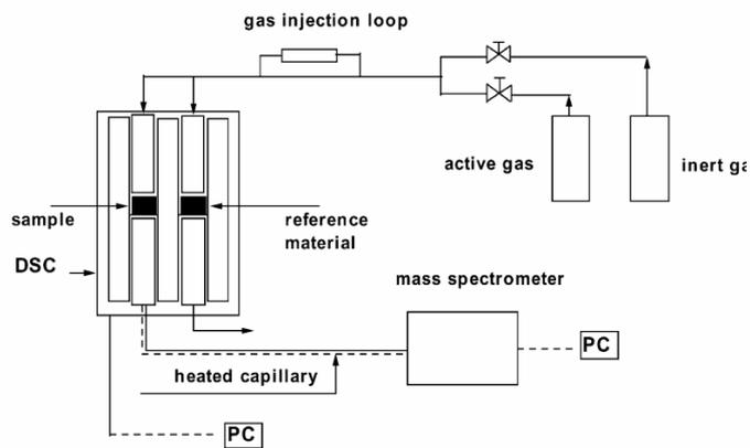
Figure 10 – Schematic representation of the Calvet type DSC with the injection loop and the MS coupling
