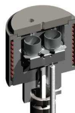
Figure 5 Cross section of a standard plate DSC
