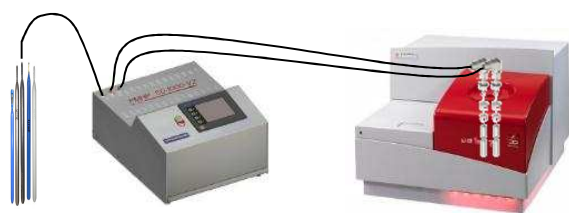
Figure 8 Experimental setting for the investigation of gas hydrates
