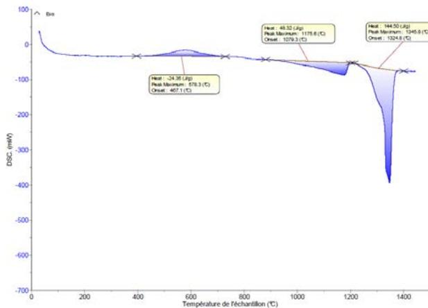
Figure 4: Heating of a Ni-CR alloy at  $10^{\circ} \text{C} \cdot \text{min}^{-1}$
