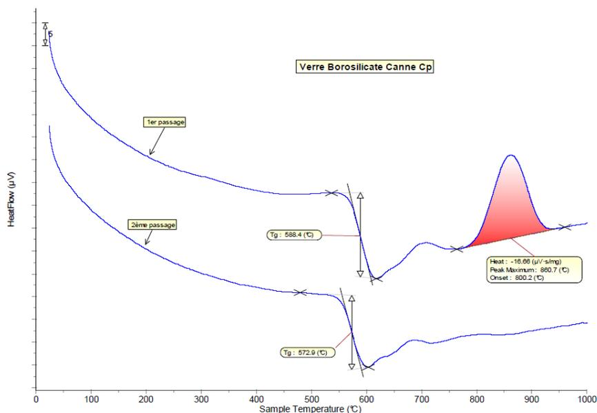
Figure 3: Glass transition and crystallization of borosilicate glass with the 3D DSC detector
