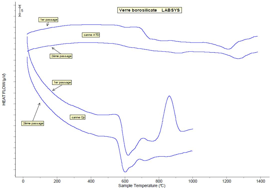
Figure 2: Investigations of borosilicate glass with the 3D DSC detector and the DTA detector
