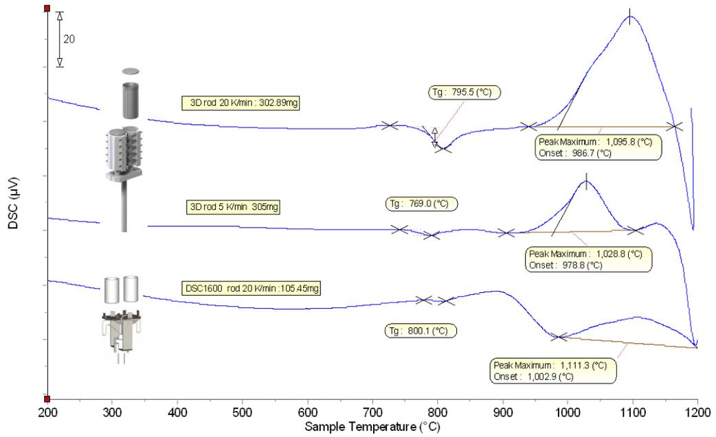
Figure 4: Glass transition and crystallization of barium based amorphous glass at 5°C.min<sup>-1</sup> and 20°C.min<sup>-1</sup>
