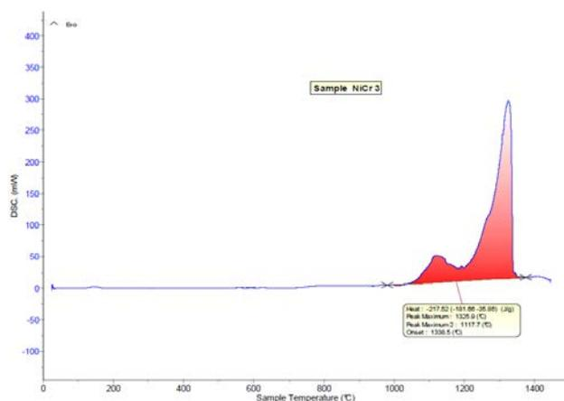
Figure 5: Cooling of a Ni-CR alloy at  $10^{\circ} \text{C} \cdot \text{min}^{-1}$
