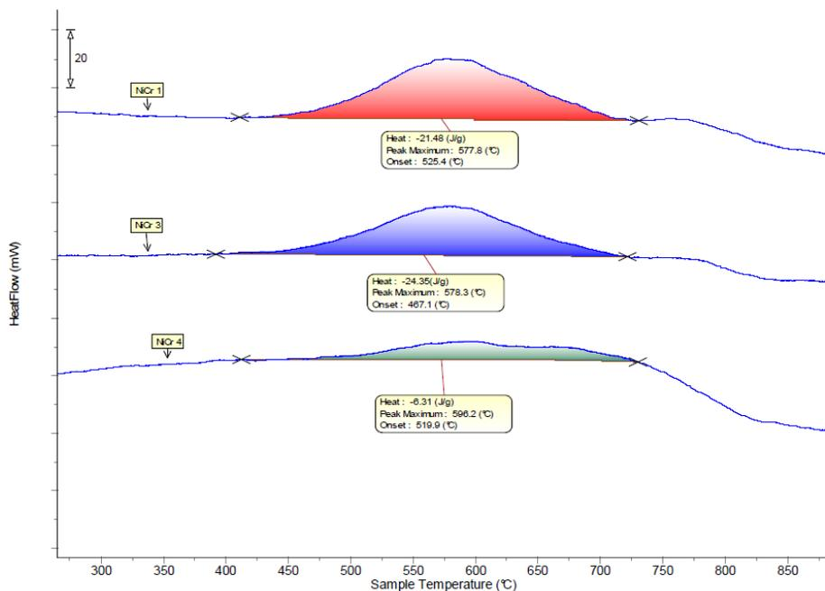
Figure 6: Crystallization of different Ni-CR alloys at 10°C.min<sup>-1</sup>
