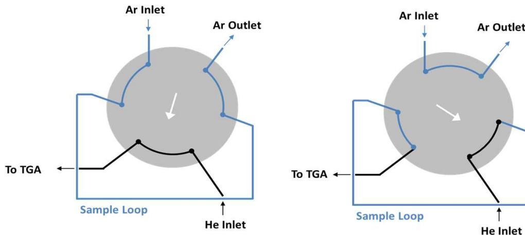
**Figure 1** – Principle of the upstream Autoinjector with dose preparation position (left) and dose injection position (right).
