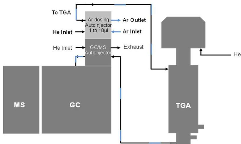
Figure 2 – Schematics of the setup with an idealized representation of the argon doses flow (blue segments).
